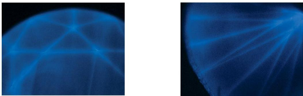
Fig. 1. “Fluorescence Cage” , A cage pattern of intense fluorescence on facet edges of Table and Pavillion of a HPHT-treated type I diamond ( from ref.1)
